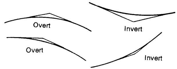
Figure 9-19. Types of vertical curves
